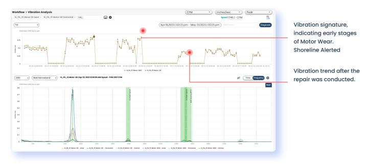
The Shoreline AI platform was able to alert the customer of an increase in the vibration trend as well as a precise analysis on where the anomaly was coming from. In this instance, it was the drive end of the motor.
